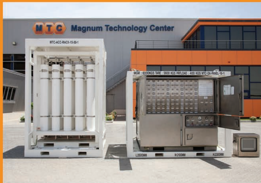
BOP/DA Panel with remote HMI and Accumulator rack in DNV frames.
