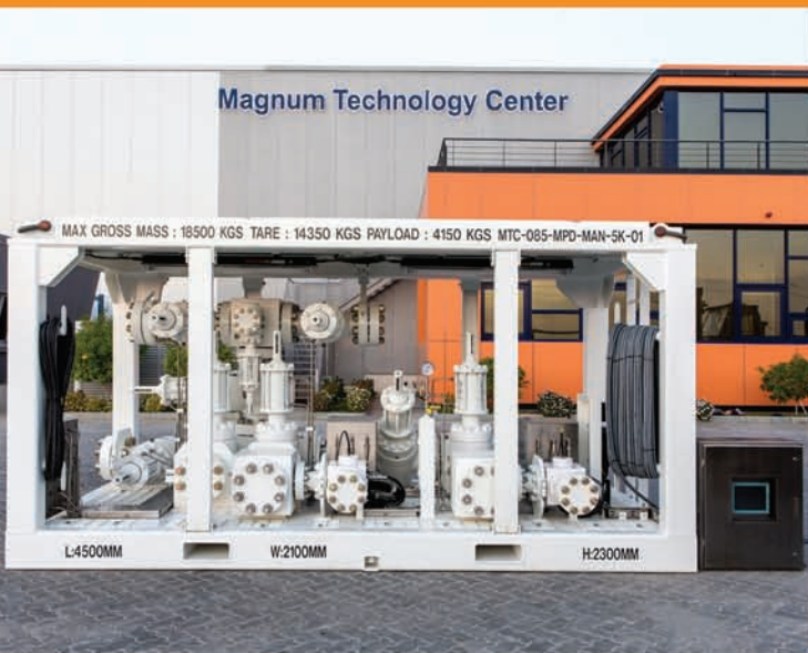
5K Managed Pressure Drilling control manifold.
